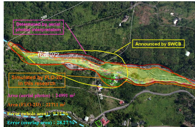
Figure 9. Comparison of debris-flow hazard zone predicted by SWCB method and presented method for the case of Hualien 072
