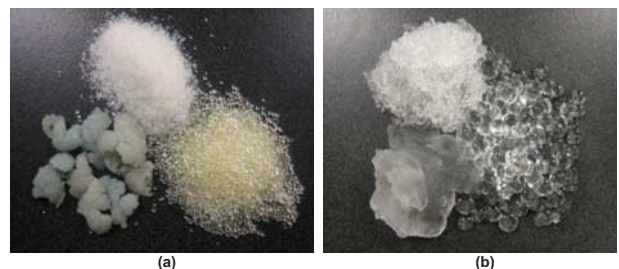
FIG. 3—Types of Aquabeads: (a) Original specimens and (b) water hydrated specimens (from left to right: C50, 200–1 %, and NC100).
