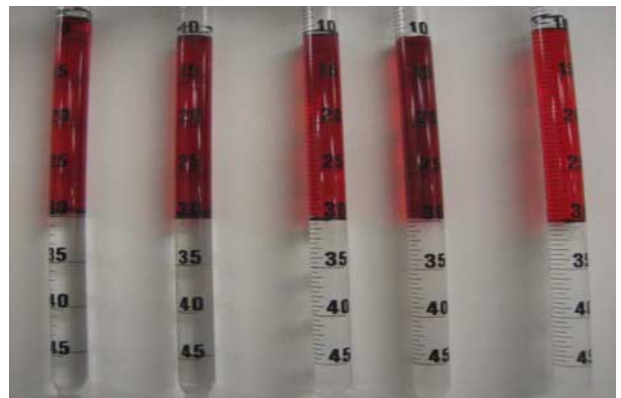
FIG. 16—Phase behavior test after equilibrium. Dark portion of the tube: Dyed mineral oil. Clear portion of the tube: Surfactant solution with different concentrations (from left to right: Triton X-100 with 0.1, 0.05, 0.025, 0.0125, and 0.006 25 % by weight).
