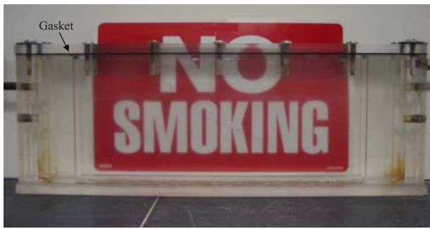
FIG. 1—No smoking sign viewed through 2.8 cm thick Aquabeads 200 in a Plexiglas mold with internal dimensions = 40 \times 2.8 \times 14.7 cm 3 .
