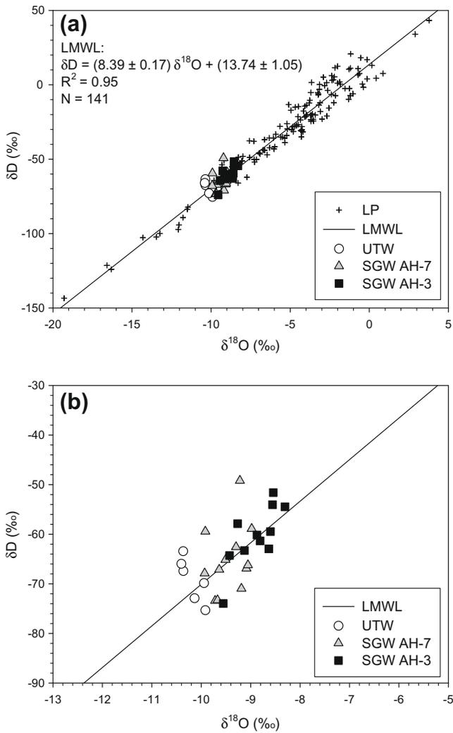
**Fig. 3.** Plot of  $\delta D$  vs.  $\delta^{18}O$  of precipitation (LP), up-tank water (UTW), and slope groundwater (SGW) samples of AH-7 and AH-3 in the slope region. The local meteoric water line (LMWL) is established as  $\delta D = 8.39 \delta^{18}O + 13.74$  by data of local precipitation.
