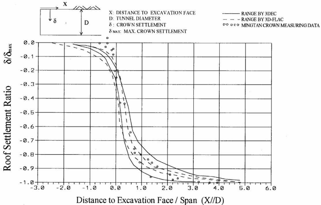
**Fig. 5 Development of tunnel movement with the advance of excavation face**
