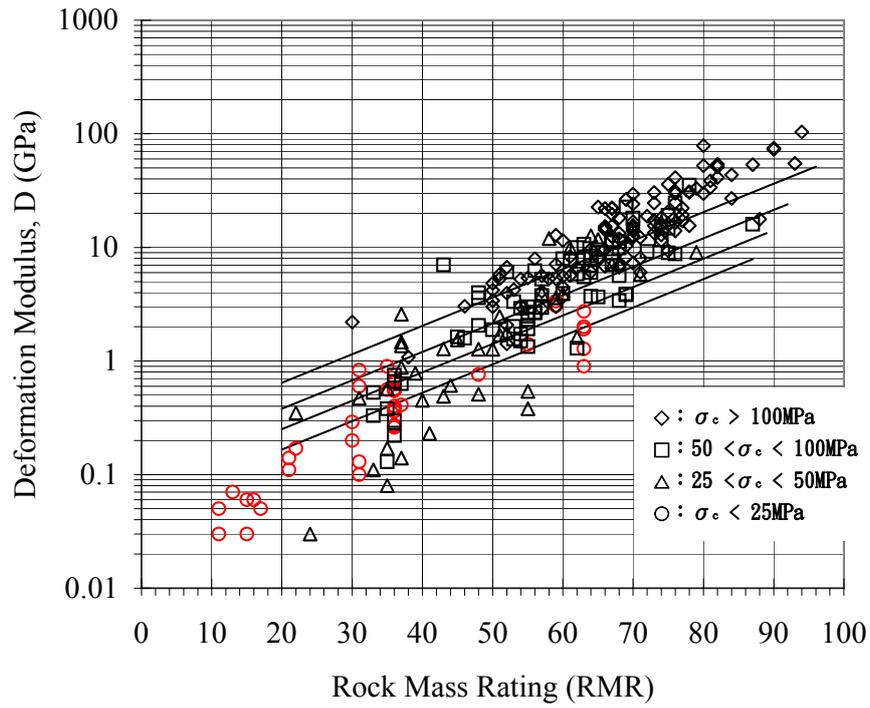
**Fig. 2 Deformation modulus of rock mass vs RMR for igneous/metamorphic rocks of various rock strengths**
