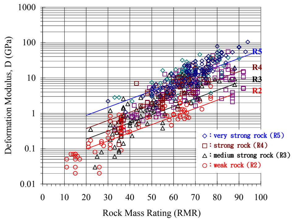
**Fig. 3 Deformation modulus of rock mass vs RMR for sedimentary rocks and igneous/metamorphic rocks of various rock strengths**
