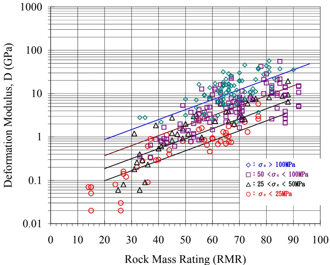
**Fig. 1** Deformation modulus of rock mass vs RMR for sedimentary rocks of various rock strengths
