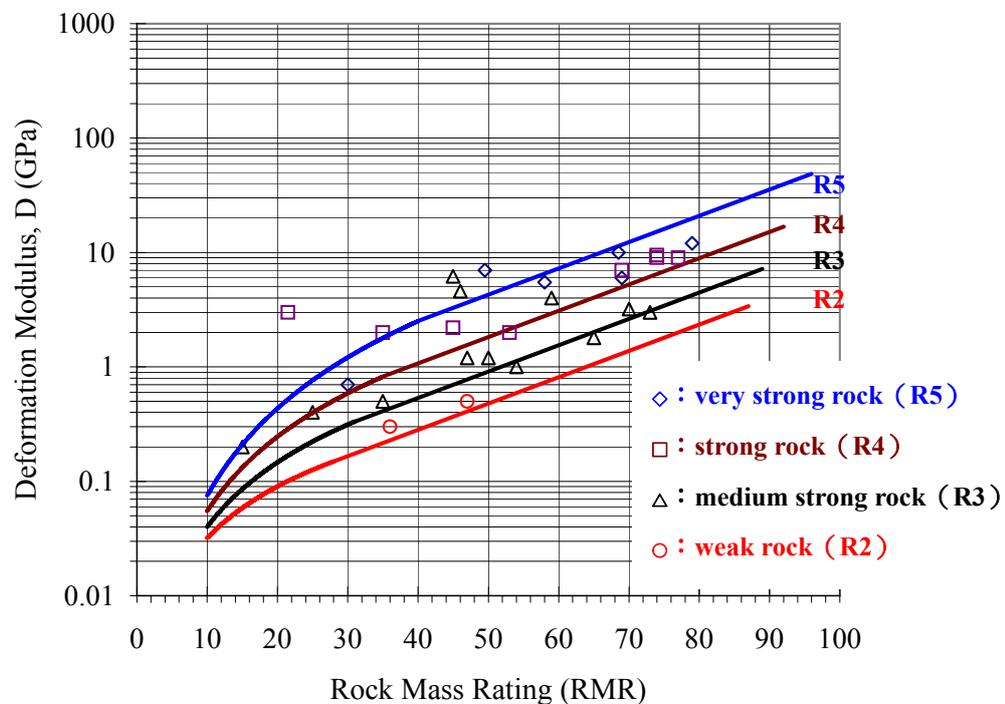
Fig. 6 Re-examination of empirical relationship by using results of back analysis of underground excavation case histories
