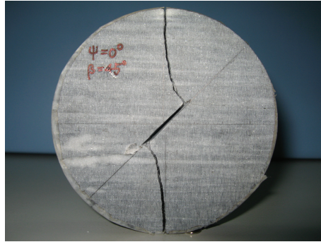
Figure 14: Photograph of specimen AM-4 after failure ( \psi = 0^\circ and \beta = 45^\circ ).
