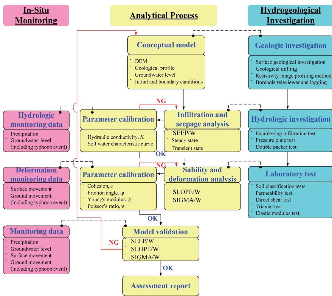
Fig. 6 Flow chart of rainfall-induced landslides hazard assessment.
