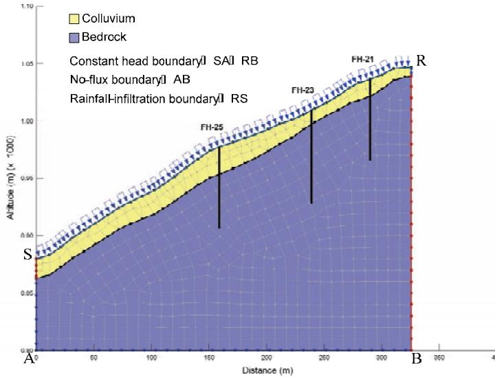
Fig. 7 Hydrogeologic conceptual model and boundary conditions of Ji-Lou study area.
