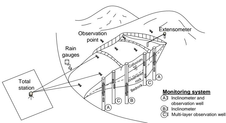
(a) Layout and design of monitoring system
