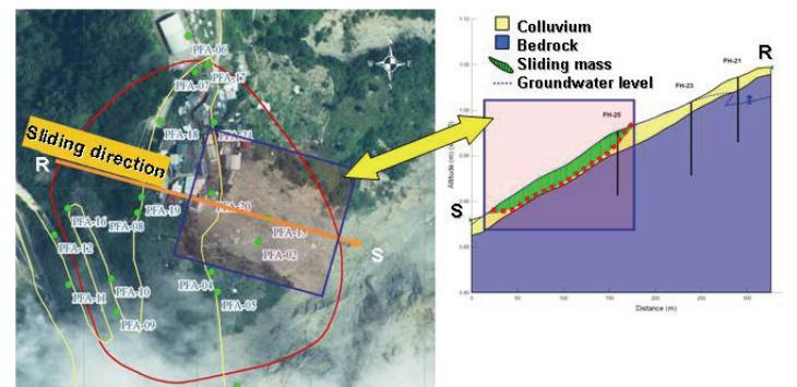
Fig. 10 The result of stability analysis compares with field condition.
