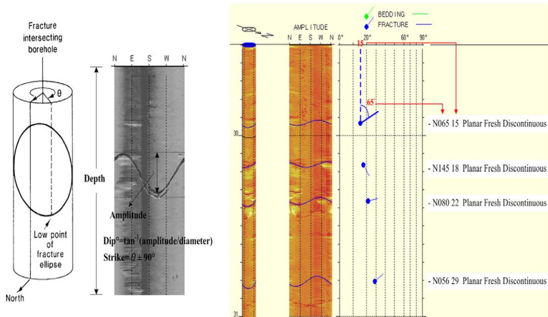
Fig. 6. Fracture strike and dip determination from televiewer logging (revised after Paillet et al., 1987) (left); and fracture orientation calculated by Rgldip 6.0 (right).
