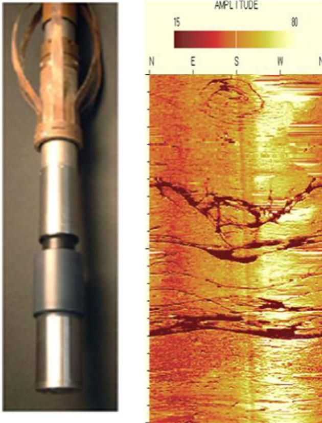
Fig. 1. Acoustic televiewer and scanned borehole image.
