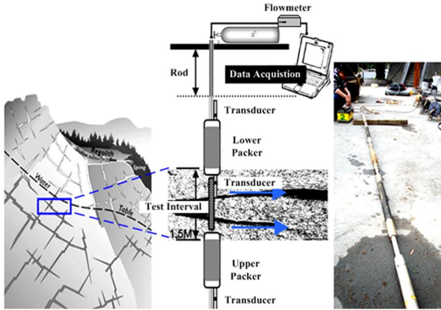
Fig. 3. Schematic drawing of double packer system.
