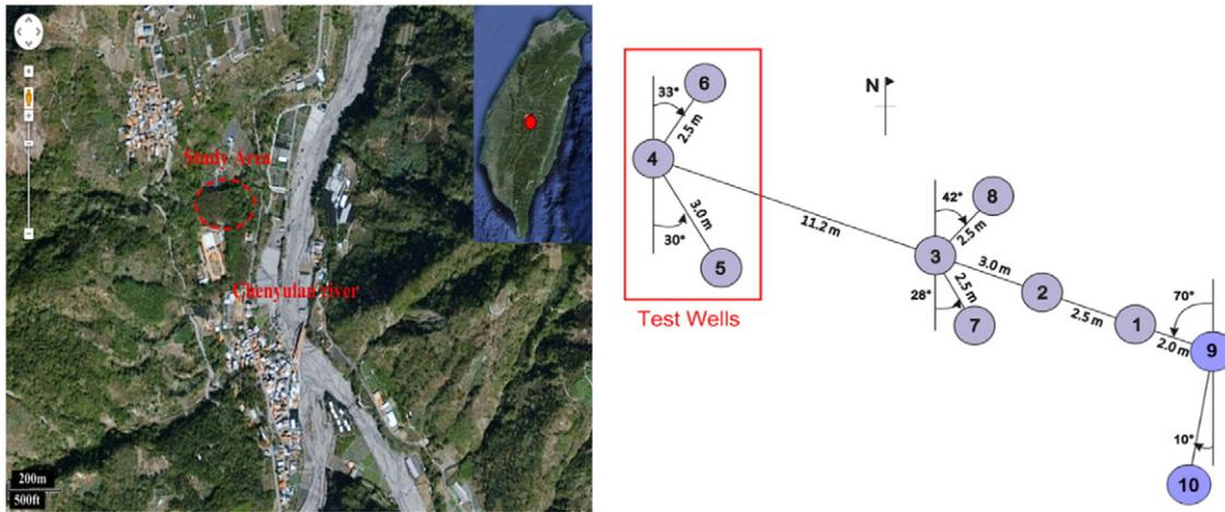
Fig. 10. Aerial photo and borehole distribution of the Hoshe test site.
