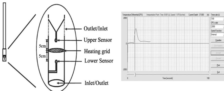
Fig. 2. Schematic drawing of flowmeter (left); and heat-pulse curve (right: the elapsed time in X-axis and the temperature difference measured by the thermistor in Y-axis) (revised after Lee et al., 2012).
