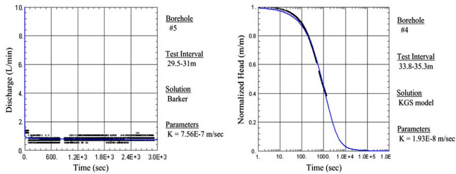
Fig. 4. The hydraulic parameters computed using AQTESOLVE: constant flow test data (left); and pressure pulse test data (right).
