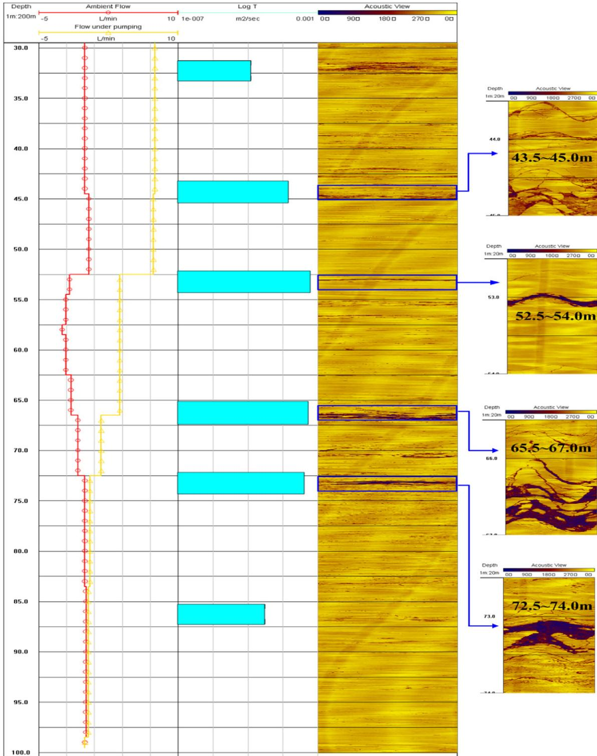
Fig. 8. Ambient and injection flow profile measured by the flowmeter; transmissivity obtained by the packer test; and borehole televiewer log of borehole EH-03.
