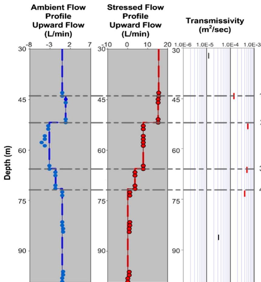
Fig. 9. Cross-comparison of flow profile required from the FLASH program (circles: measured data; line: simulated results) and transmissivity of borehole EH-03.
