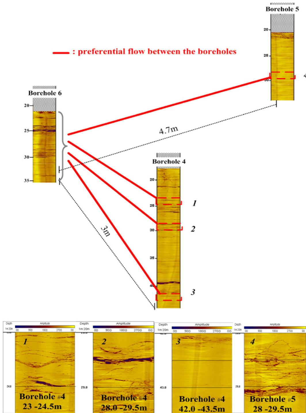
Fig. 14. Schematic drawing of preferential flow between the boreholes in the Hoshe test site.
