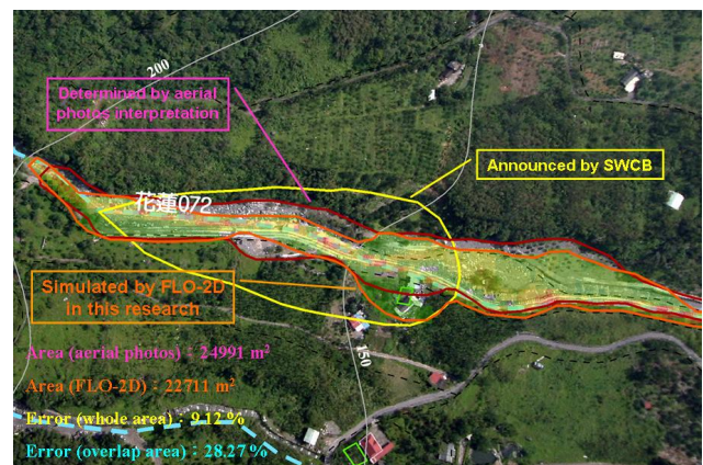
Fig. 13. Comparison of debris-flow hazard zone predicted by SWCB method and presented method for the case of Hualien 072.
