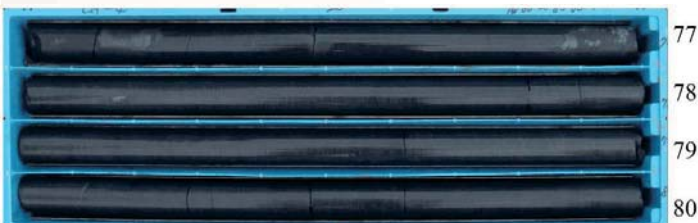
Fig. 2(b). Rock core photos of borehole CH-04 without fault influence.
